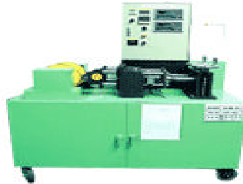
Reliability Testing Apparatus for Escalator Step roller, Guide roller and Parking system roller
